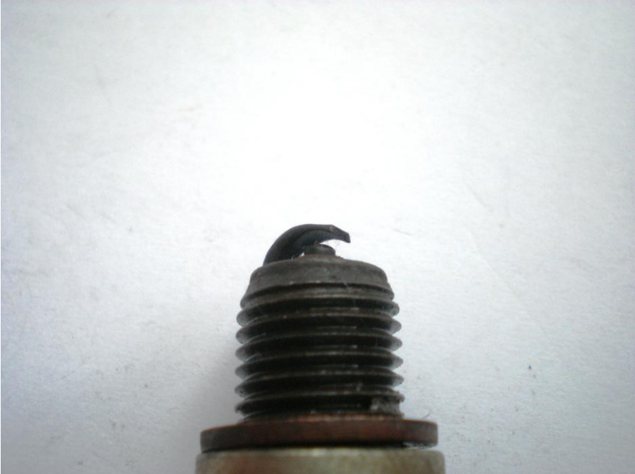
Fig. 3 - Spark plug used, evaluated visually as worn out
