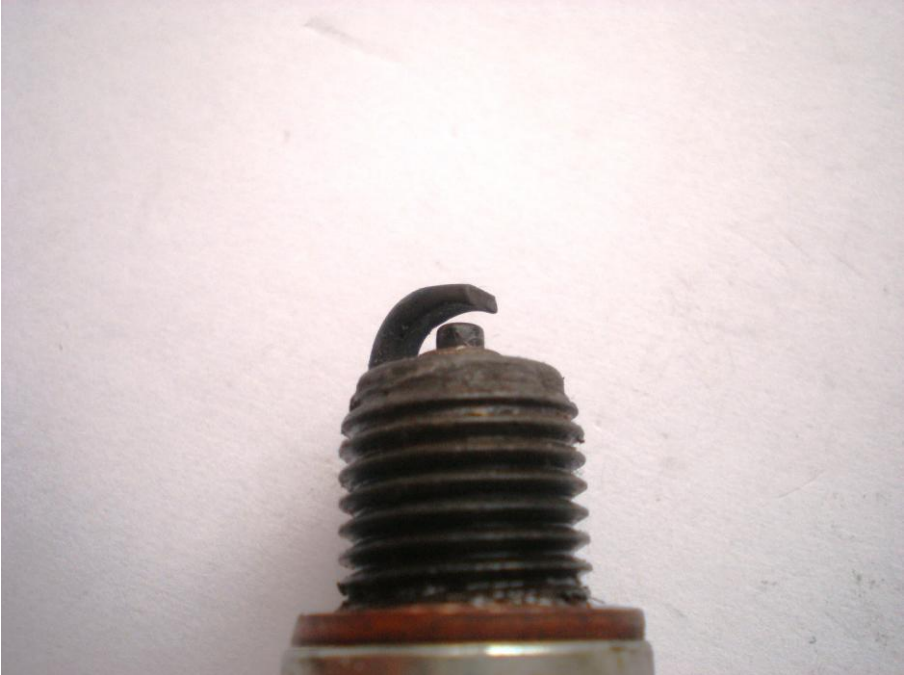
Fig. 2 - Spark plug used, evaluated visually as good prior to electrode adjustment
