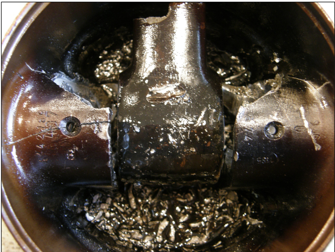
Fig. 3 – Fatigue fracture of the piston pin boss
