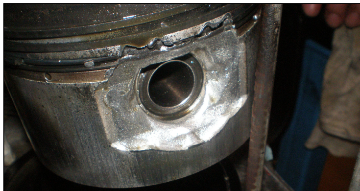
Fig. 1 – Piston side spoiled by the cleared locking snap ring (p/n Sc2515).
