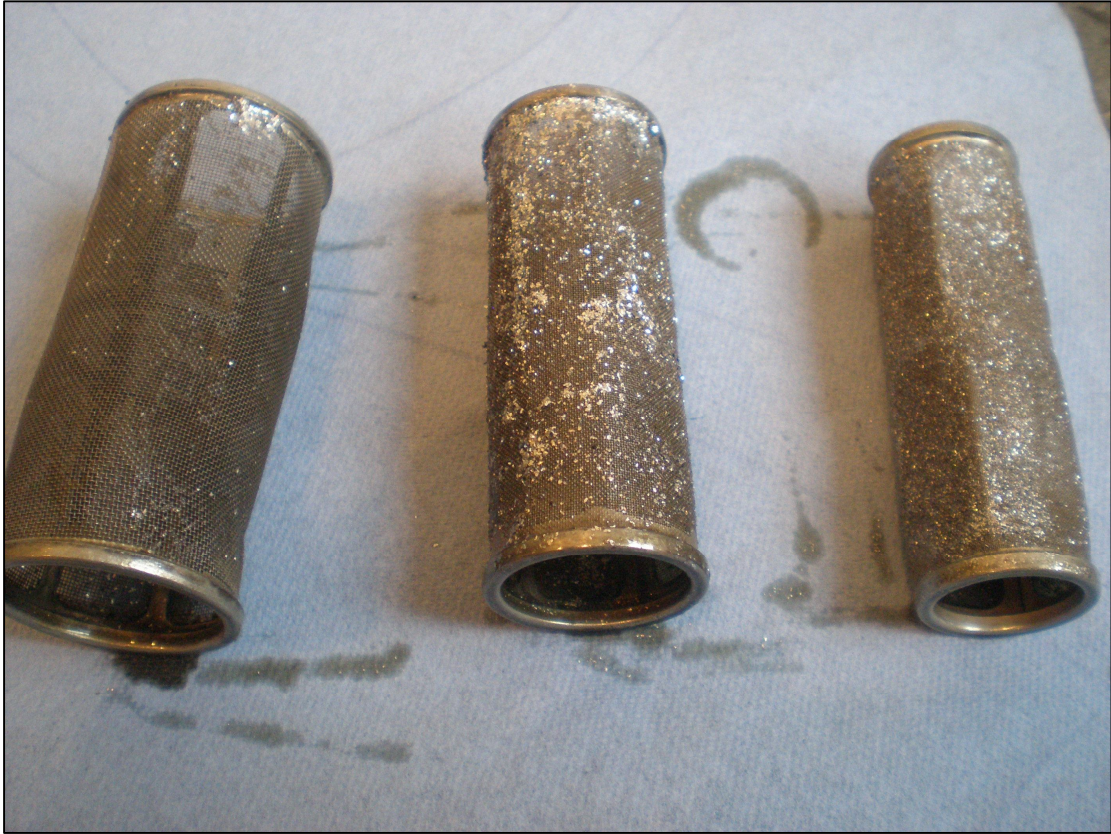
Fig. 2 – Aluminum alloy chippings on the three stages oil strainer filter (chippings origin is the piston)
