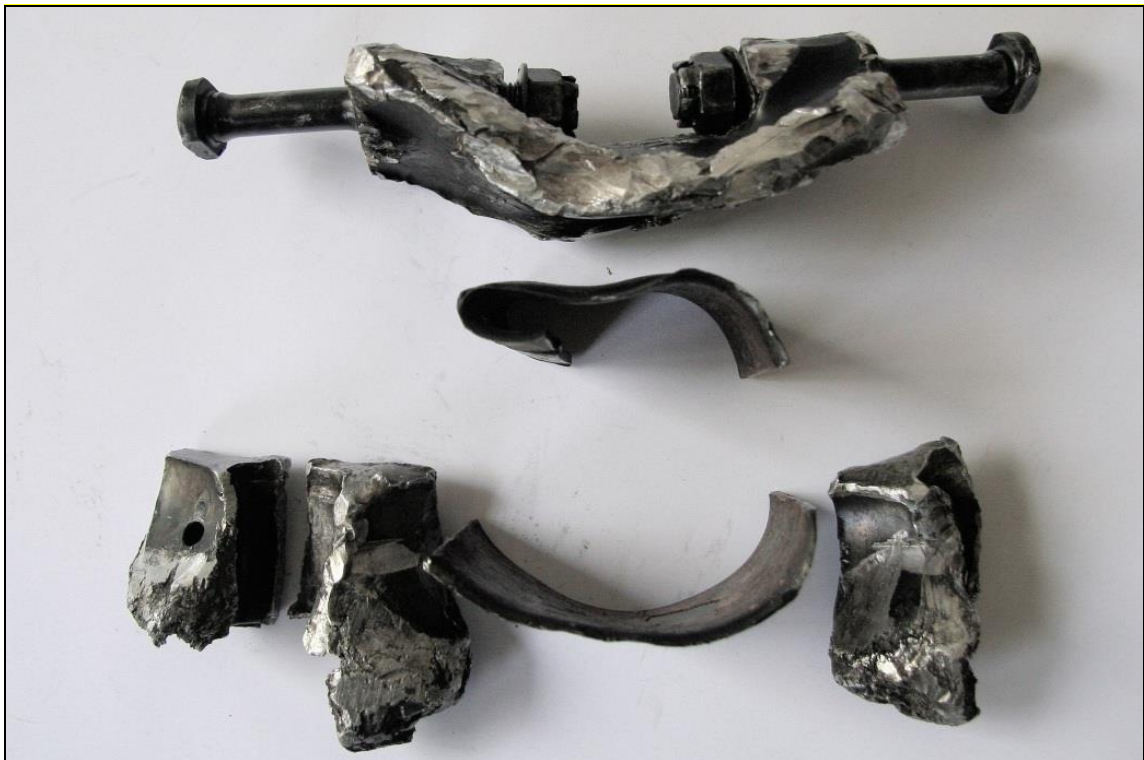
Fig 2 – Big end upper half No. 6 fragments and deformed big ends bearing.
