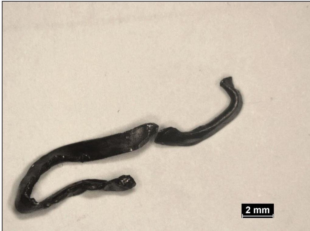
Fig 5 – Fragments of the cotter pins belonging to the bolts of the connecting rod No. 6.
