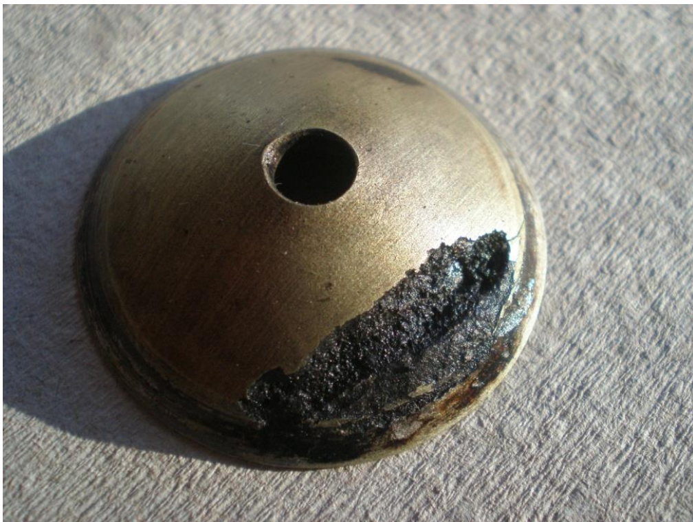
Fig 8 – Plug from crankpin No. 6, bottom view. Significant wall wearing by the corrosion affecting.
