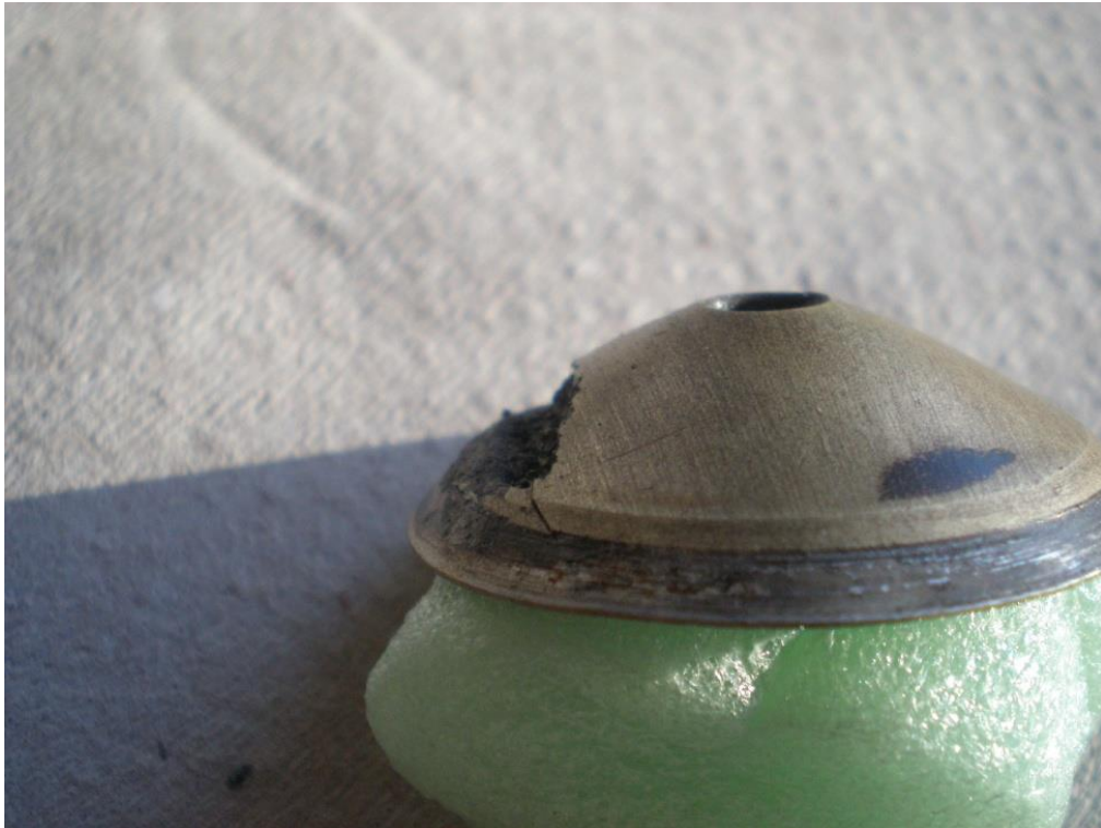
Fig 7 – Plug from crankpin No. 6, side view. Significant wall wearing by the corrosion affecting.
