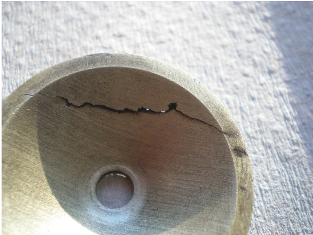
Fig 9 – Crack at the area of the wall wearing on the opposite surface compare to these shown on the Figs 7 and 8 ones.
