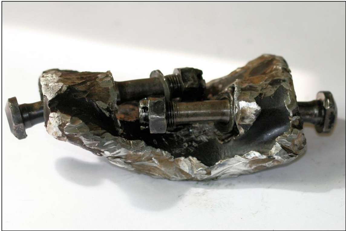
Fig 3 – Detail = Deformed big end lower half No.6 and locking bolts w/ female nuts without cotter pins.
