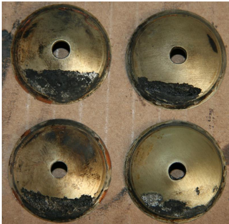
Fig 6– Corrosion of the crankpins holes plugs, upper part = plugs from crankpin No. 6, lower part = plugs from crankpin No.1 (referential).
