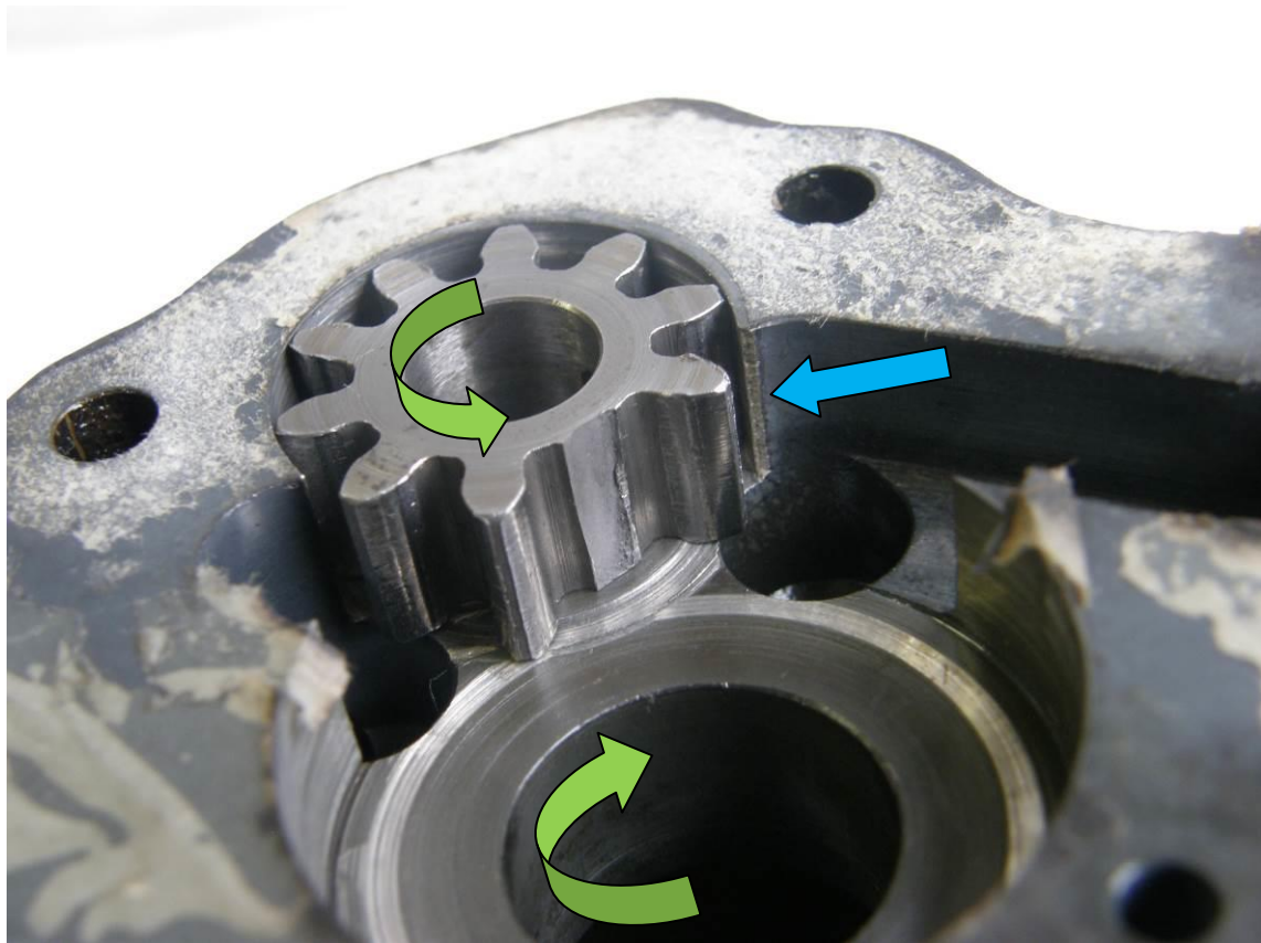
Fig. 2 – The scavenge oil pump of the M137AZ cam housing with worn-down teeth and abraded edge of the chamber, the green arrows indicate the direction of rotation of the gear, the blue arrow points to the edge of the chamber abraded by the gear burrs.
