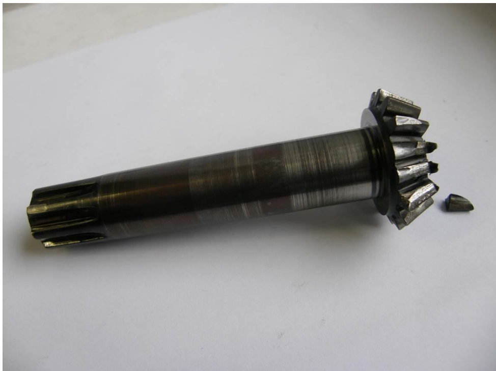
Fig. 4 – The damaged p/n Sc3755 gearwheel with a broken off tooth.
