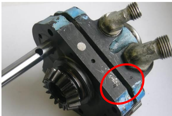
Fig. 1 – The material damaged scavenge oil pump of the cam housing, set No. 4.
