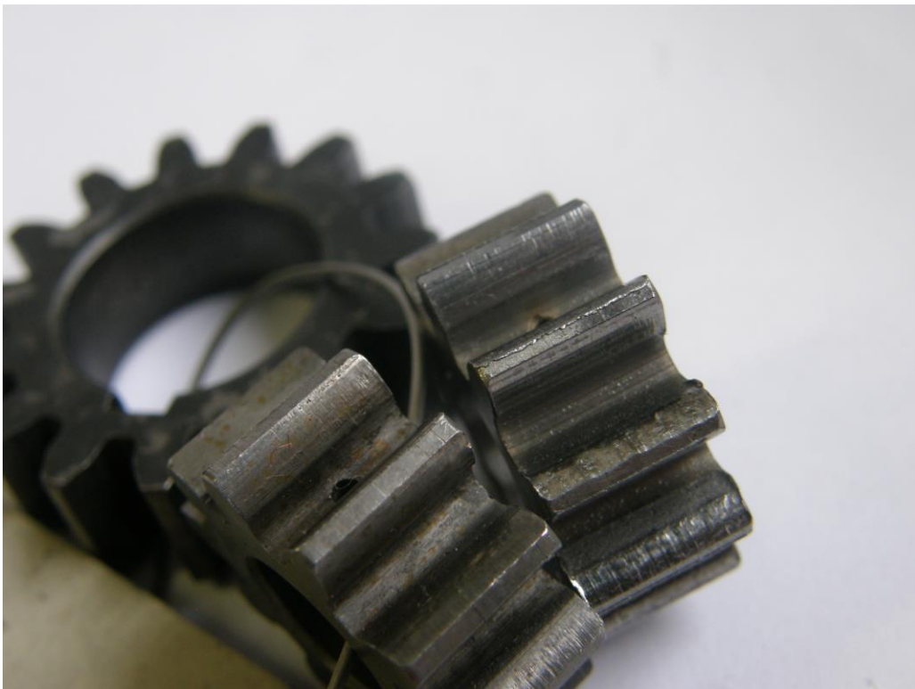
Fig. 7 – Comparison of the gearwheel after 1,400 hours of operation (left) and the damaged gearwheel of unknown origin (right).
